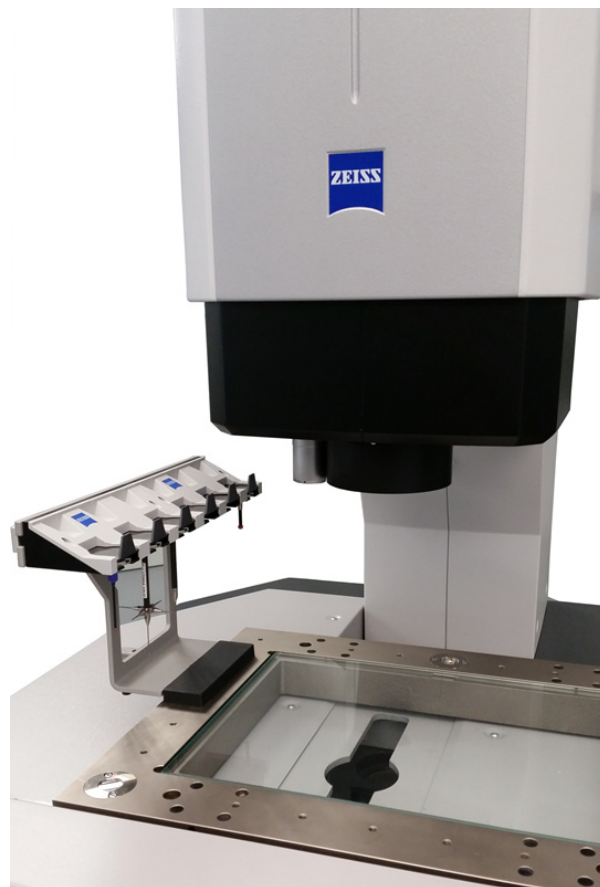
Fig. 3: MSR O-INSPECT installed on the CMMs
